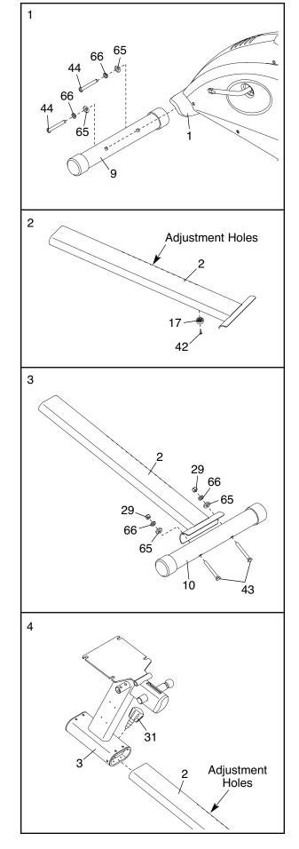
4. Orient the Seat Carriage (3) as shown. Slide the Seat Carriage onto the Seat Rail (2), and then tighten the Seat Carriage Knob (31) into the Seat Carriage and an adjustment hole in the Seat Rail. Make sure the Seat Carriage Knob is engaged in one of the adjustment holes.
